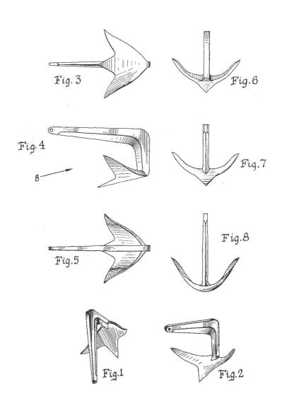
FIG. 1 and FIG. 2 are perspective views of an anchor showing my new design;
